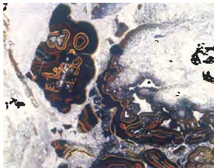
Figure 9.14 Microscope picture in transmitted light of zinc ore (sphalerite) from Galmoy mine, Co. Kilkenny.
