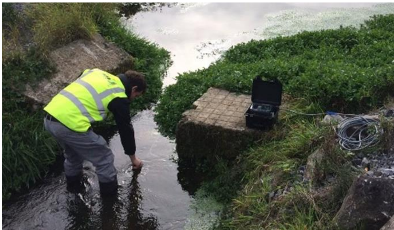
Figure 1 Deploying the GGUN-FL30 field fluorometer at Polecats Spring, Co. Roscommon
