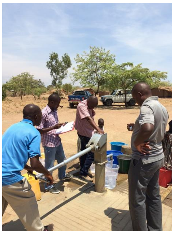
Figure 3 Modified discharge test in operation, Malawi 2015 ©NERC
