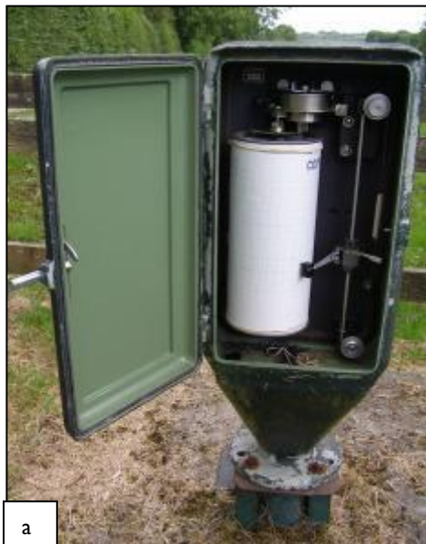
Updating groundwater level monitoring systems (a) GSI chart recording groundwater levels and (b) downloading groundwater level data from a data logger at an EPA monitoring point
