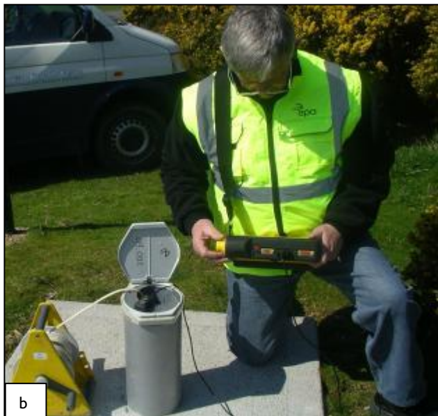
Updating groundwater level monitoring systems (a) GSI chart recording groundwater levels and (b) downloading groundwater level data from a data logger at an EPA monitoring point
