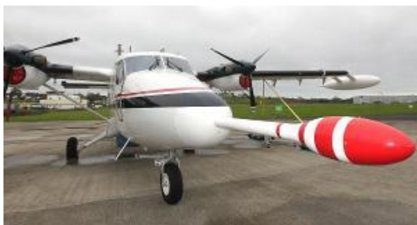
The airborne survey aircraft, a De Havilland Twin Otter operated by Sander Geophysics Ltd of Ottawa, Canada. The magnetometer is in the foreground on the nose cone and the EM coils are on the wingtips.
