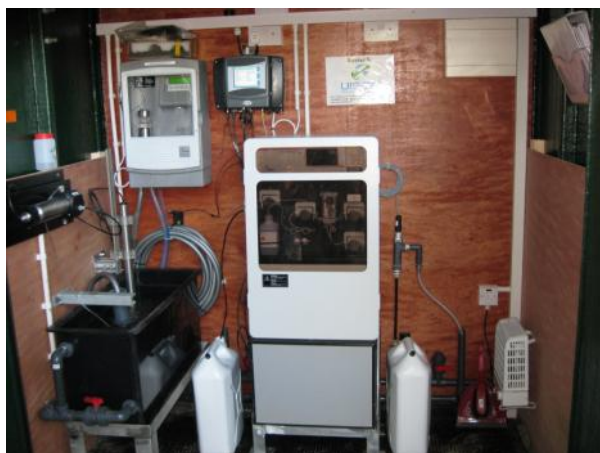
Figure 1. One of six ACP water quality stations with equipment measuring P and N fractions, turbidity, conductivity and temperature on a sub-hourly basis
