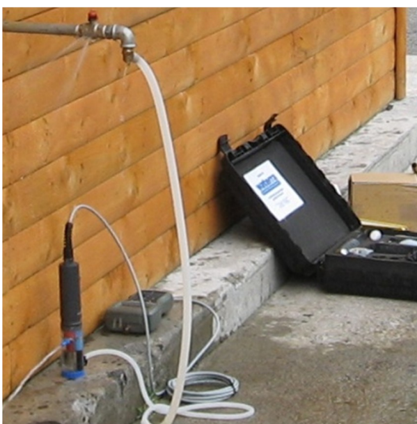
Photo 1. Sampling field parameters using a flow through cell
