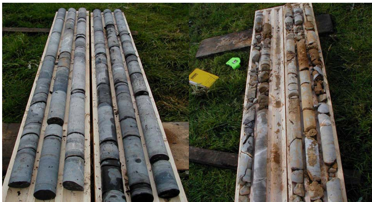
Plate 1: Mewlaghmore 1 Showing 100% recovery with clean fractures
