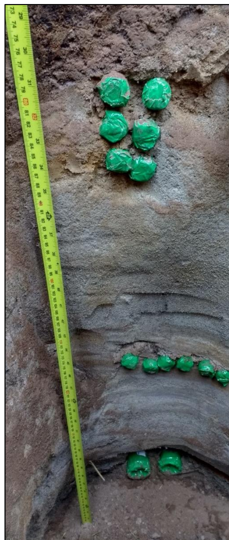
Figure 8 Photo inside trench showing equivalent dose samples for OSL analysis captured in PVC and steel tubes.
