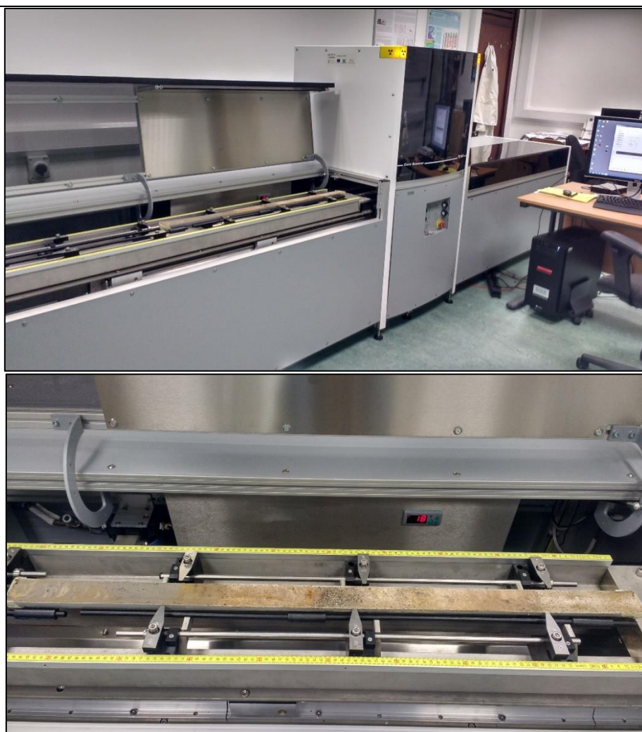
Figure 5 Sediment core in the Itrax core scanner, located in the UCD School of Geography.
