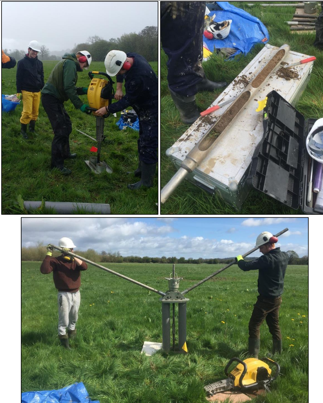
Figure 4 Sediment coring using a Van Walt percussion auger, gouge and extraction kit in the field.
