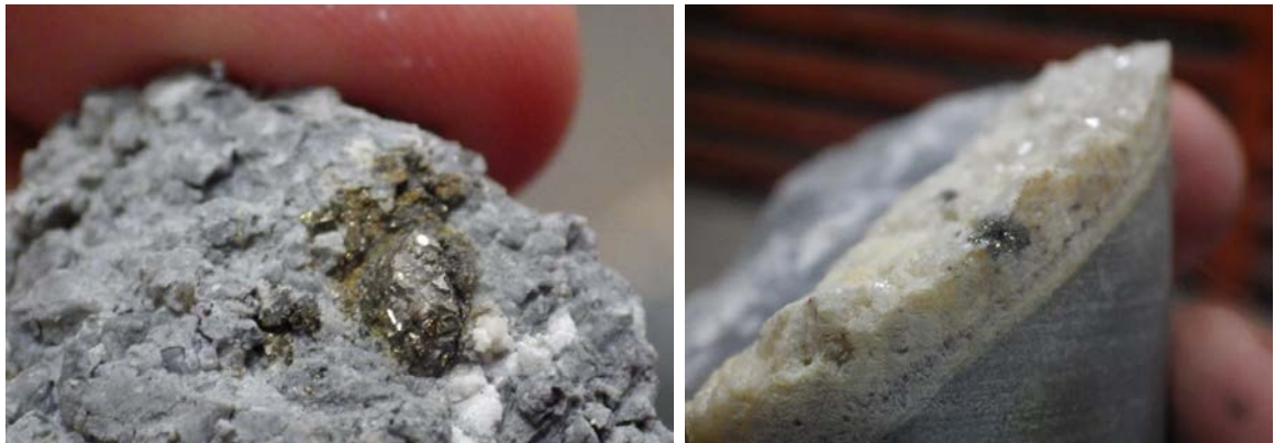
Figure 2. Selected images of sulfide minerals within fault gouge material containing micro-veins of calcite (left) and within individual calcite veins (right) at 54 m and 27 m depths of the Faughart core respectively.
