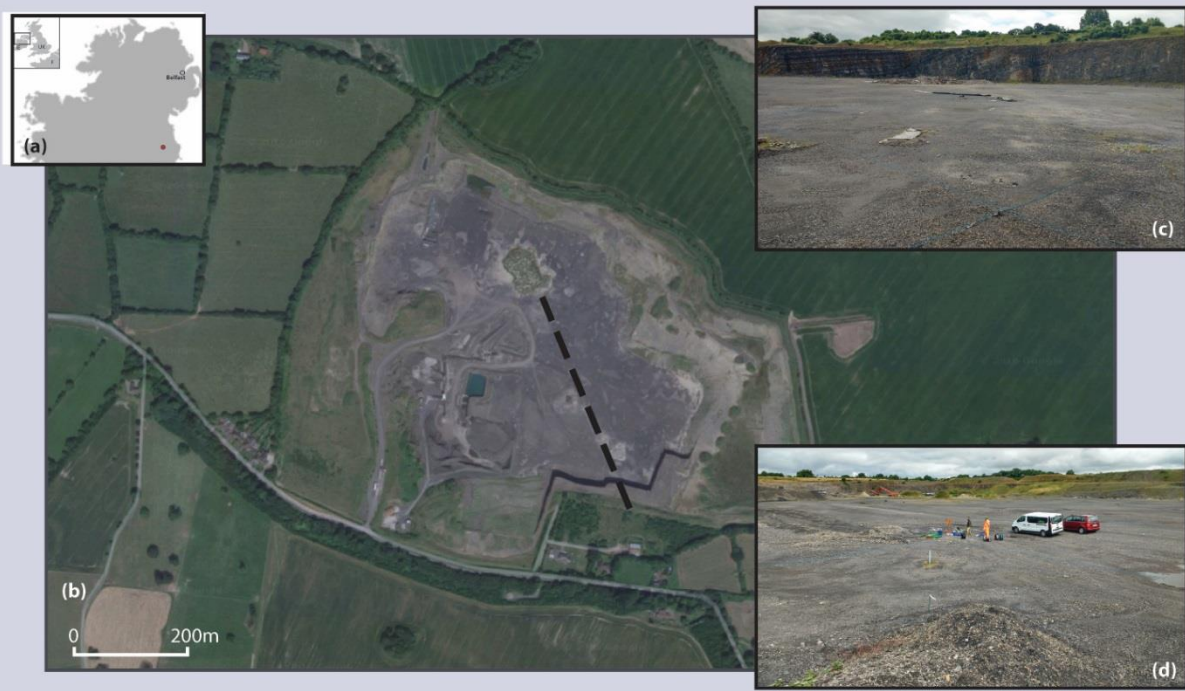
Figure 5: (a) Location of Study Site; (b) Aerial Photograph of Quarry and inferred location of fault zone (dashed line); (c) Site View of MRS Survey within Quarry (View SE along fault zone); (d) Site View of MRS Survey within Quarry (View NW along fault zone)
