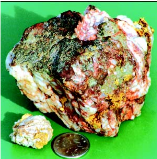
Figure 1. Sample with gold from West Wicklow (photograph courtesy of Exploration and Mining Division, Department of Communications, Marine and Natural Resources). Arrows point to the visible gold.
