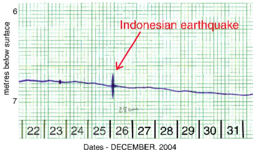
All three wells simultaneously registered abrupt water level changes in the early hours of 26 December 2004 (the chart does not allow the precise time to be registered). The maximum fluctuations ranged from about 50 mm in 18/92, to 240 mm in 25/78, to 280 mm in 31/72. The differences are probably related to the differing storage coefficients in the three aquifers - the gravel aquifer will have the largest storage coefficient, giving the lowest response to a given pressure.
