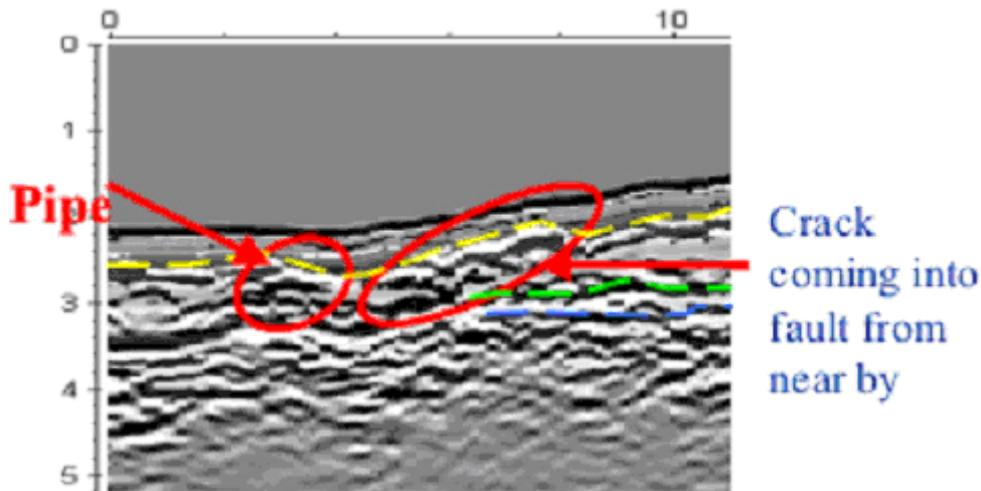
Ground Penetrating Radar image from Shane Murphy's work, showing interpreted "pipe" and "crack" features which may be important in initiation and localisation of peat failures
